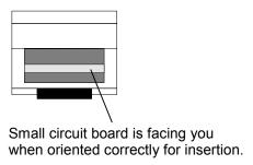
Figure 6-16 End View of Small Form Factor Pluggable Transceiver
